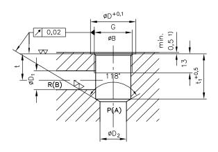
1) A counter bore of 0.5 mm is required, if the pressure at R exceeds 100 bar!
