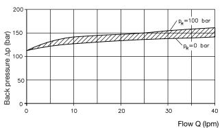
Viscosity during measurements approx. 60 mm<sup>2</sup>/s
